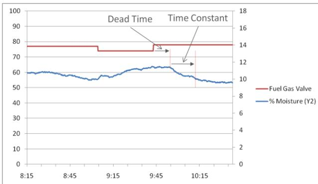
Figure 4. Dryer step test data showing controller output changes and their effect on DDG moisture.
