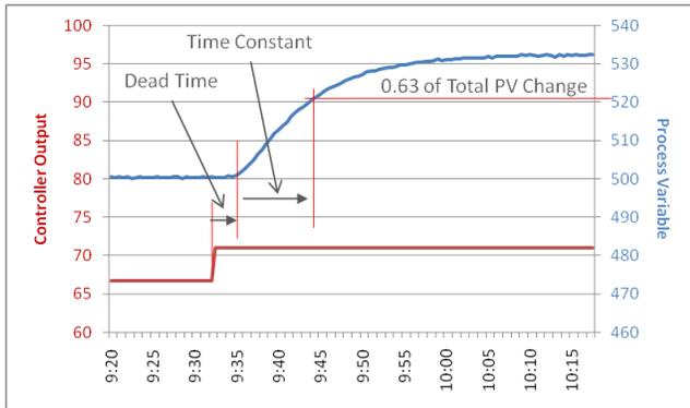
Figure 3. Example of process characteristics for tuning.
