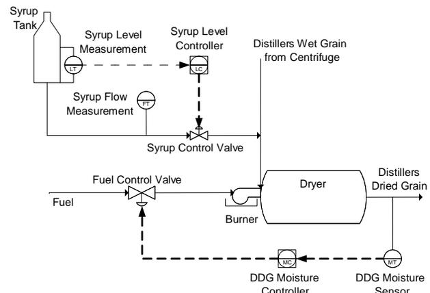
Figure 1. DDG moisture and syrup level control loops.
