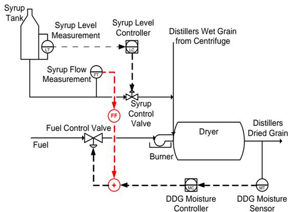
Figure 6. Feedforward controller.
