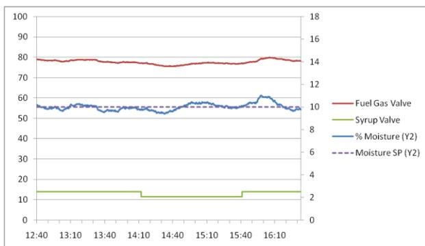
Figure 7. Improved moisture control with feedforward.
