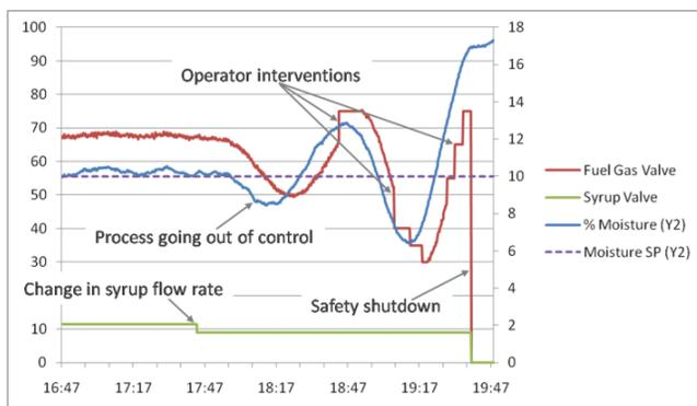
**Figure 2. Unstable moisture control after changing syrup flow rate.**
