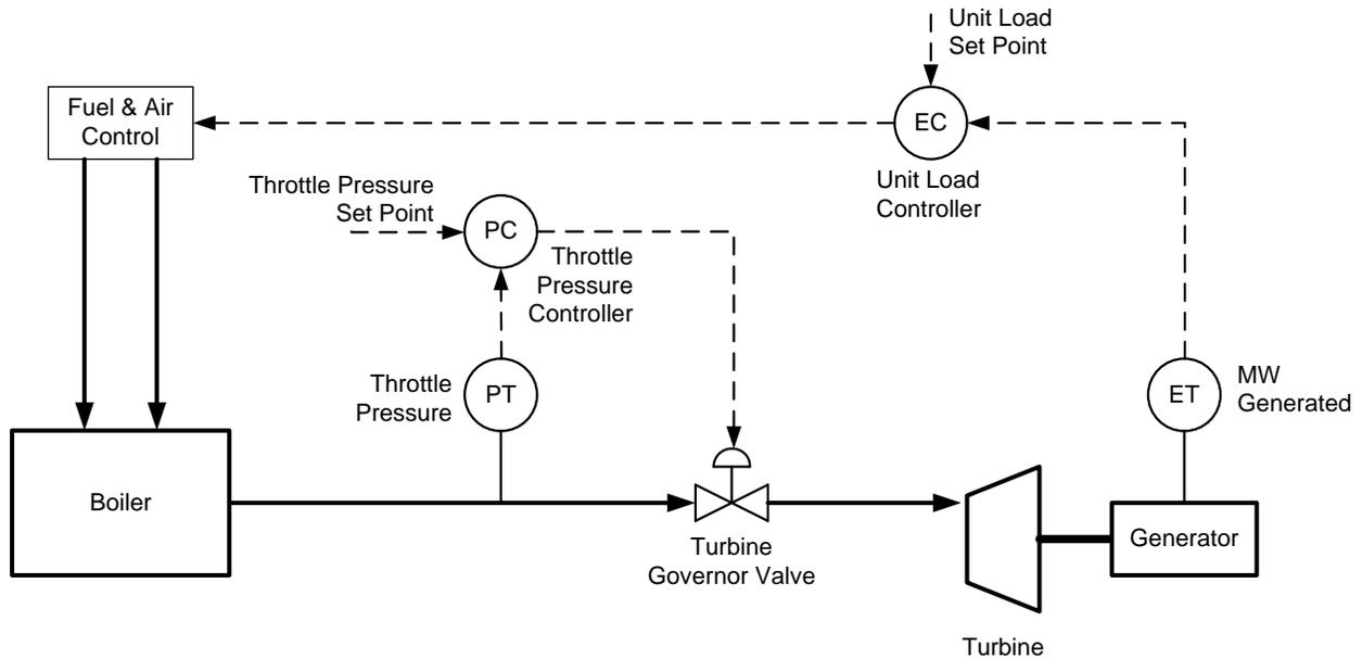
**Figure 3** In turbine-following mode the throttle pressure is controlled by the governor valves and MW produced is controlled by the firing rate of the boiler.
