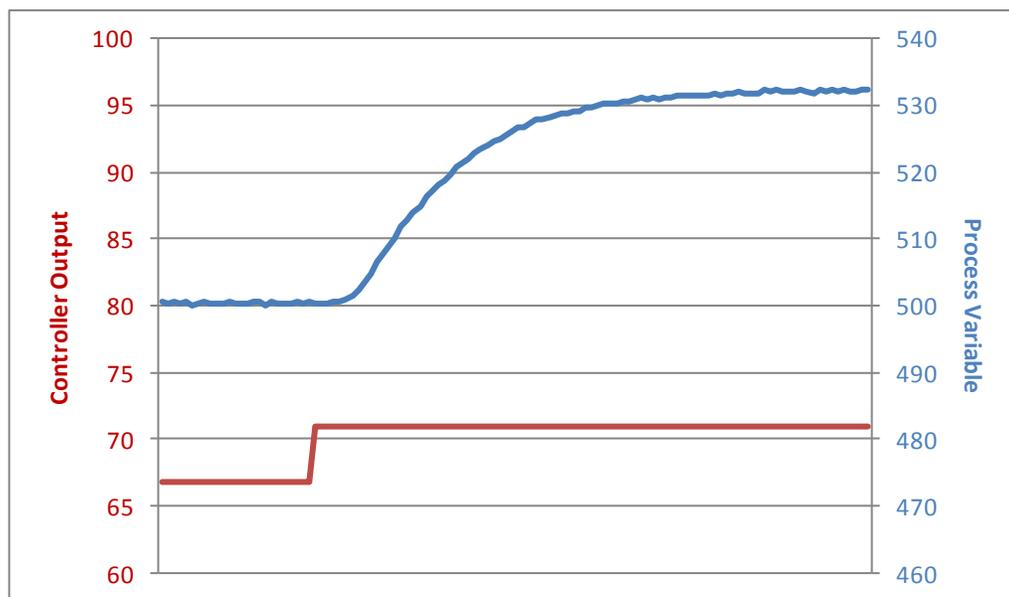
Figure 1 Step-response of a self-regulating process.
