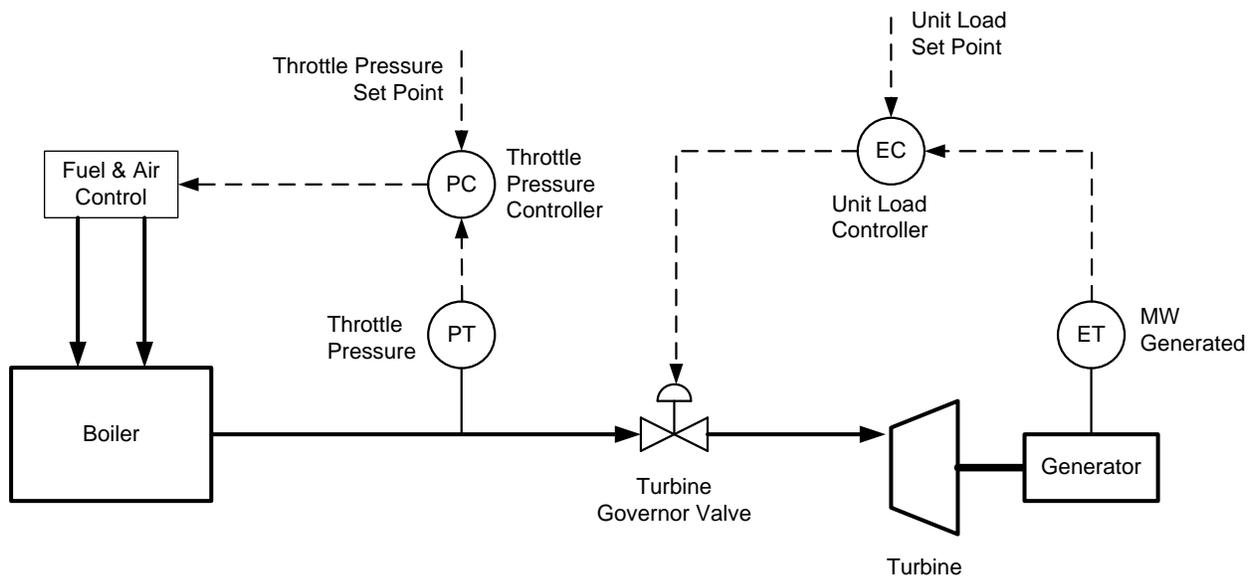
**Figure 5** Boiler-following mode the throttle pressure is controlled by the firing rate of the boiler and MW production is controlled by the governor valves.
