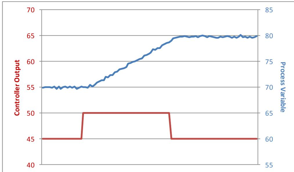
**Figure 2** An integrating process stabilizes only after the controller output is returned to its original level.
