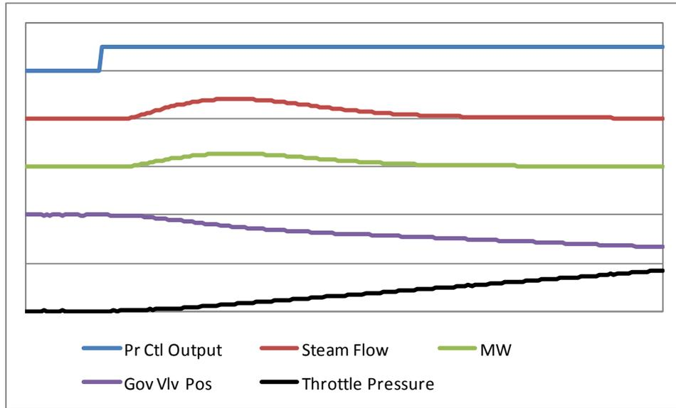
**Figure 6** In boiler-following mode, the load controller throttles down the governor valves to control MW after a change in throttle pressure controller output, causing the throttle pressure to increase like an integrating process.
