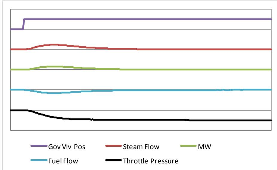
**Figure 4** In turbine-following mode, throttle pressure decreases like a self-regulating process after a step change in governor valve position.
