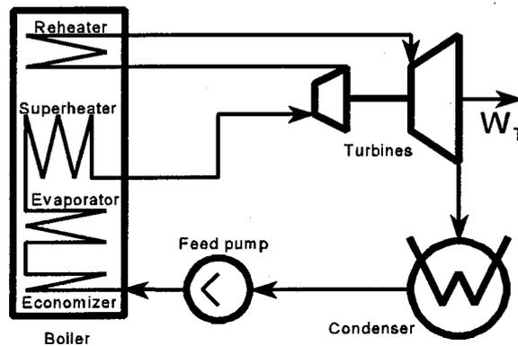
Figure 3. Power plant steam/water cycle.
