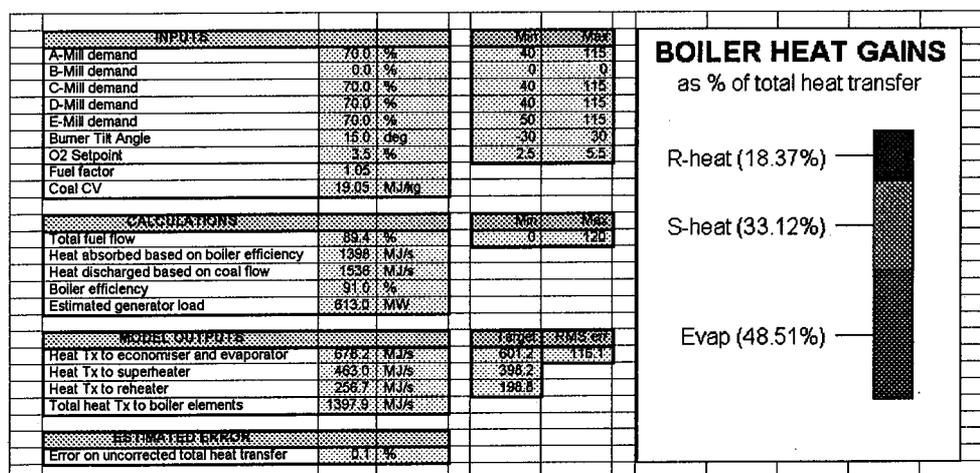
**Figure 5.** The neural network boiler heat transfer model running on a spreadsheet.
