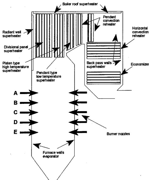
Figure 4. Typical layout of boiler elements.
