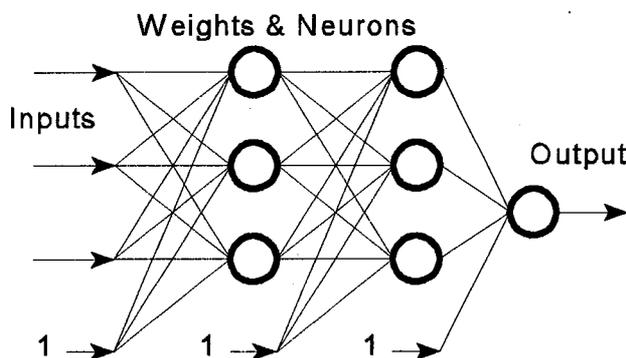
Figure 2 A small multilayer neural network.
